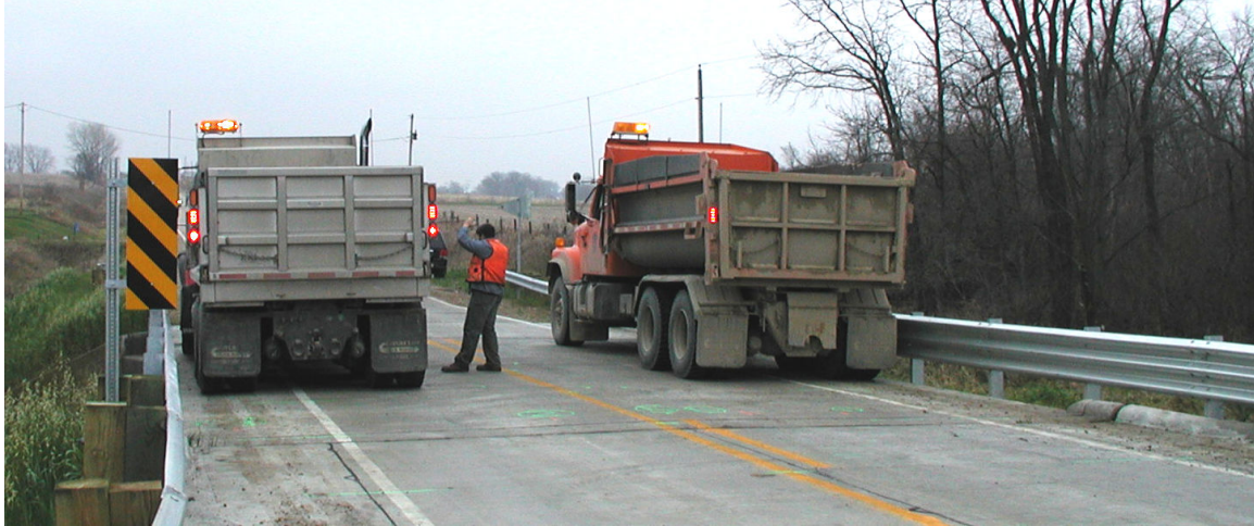
Figure 2.10. Load Case 1 (stationary) during Test 1.
